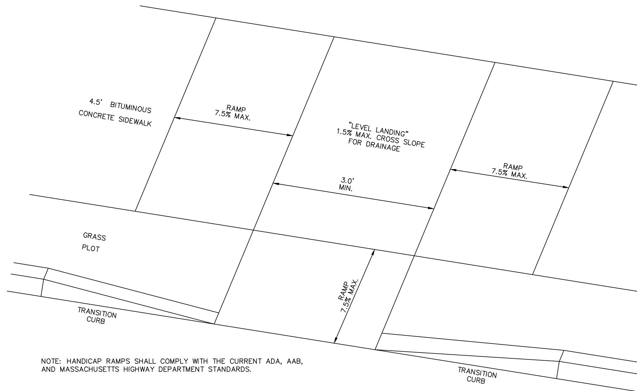
TYPICAL WHEELCHAIR RAMP DETAIL NOT TO SCALE
